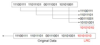
Longitudinal parity was initially used for magnetic tapes to supplement vertical parity error detection.
