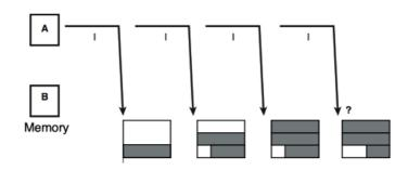
Flow control is used to set up a mechanism to control the rate at which information is sent to the receiver. It can be achieved by several methods :
