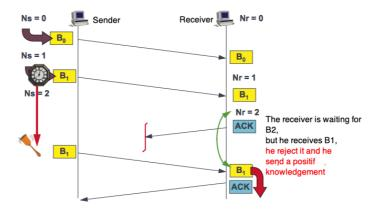
In cases where consumption delays are longer, the data may not be acknowledged on time. For example, if A transmits a block B0 and B delays in its processing, A will retransmit B0 before receiving the acknowledgment. If A transmits a new block B1 and is lost, it will consider the acknowledgment of the second B0 as an acknowledgment of B1.
