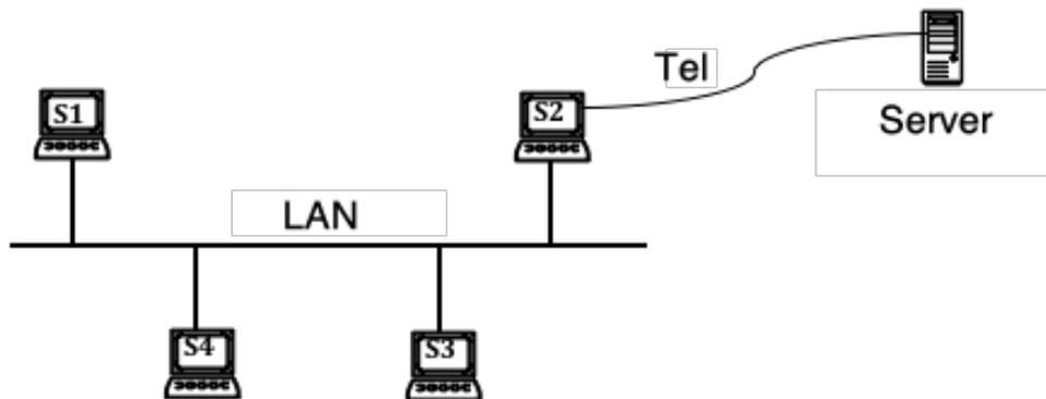
Stations  $S_1$ ,  $S_2$ ,  $S_3$ ,  $S_4$  are linked by a local bus network offering a throughput of 10 Mbits/s. The station  $S_2$  is connected to an Internet access server by a phone link whose frequency band is [300-3400 Hz]. Given that the line rate is 62 Kbits/s :
